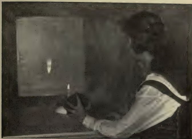
FIG. 86. The concave mirror forms an image of the burning candle.
